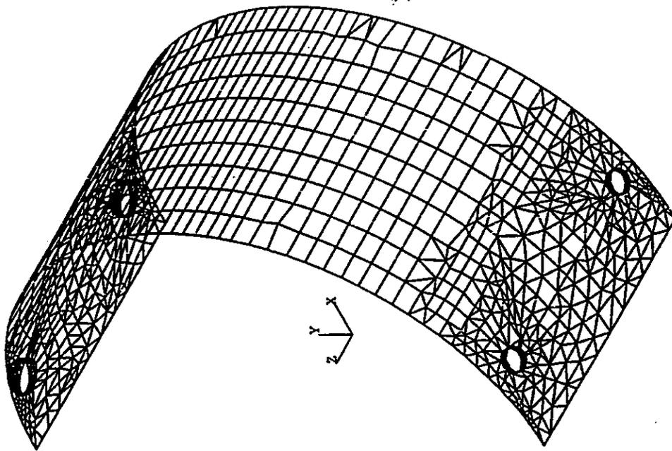
Figure 3-15 Finite Element Model for a CANDU Reactor Calandria Shell
