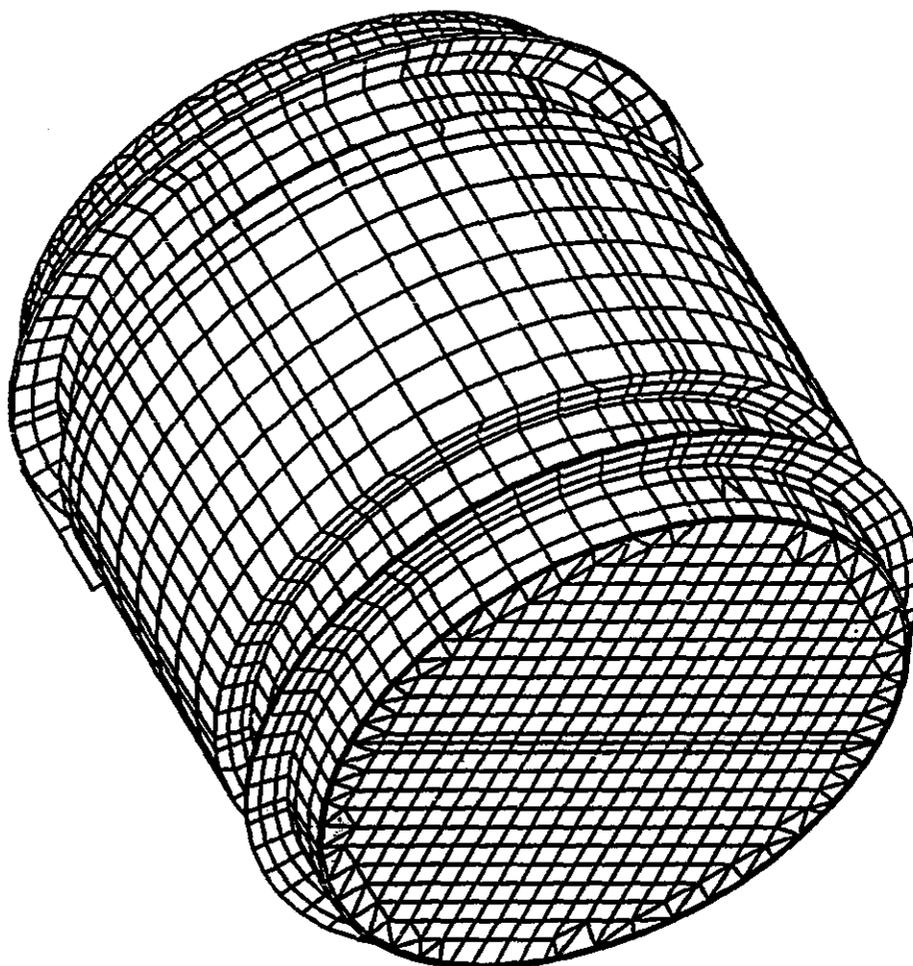
Figure 3-17 Seismic Finite Element Model for a CANDU Calandria Structure Assembly
