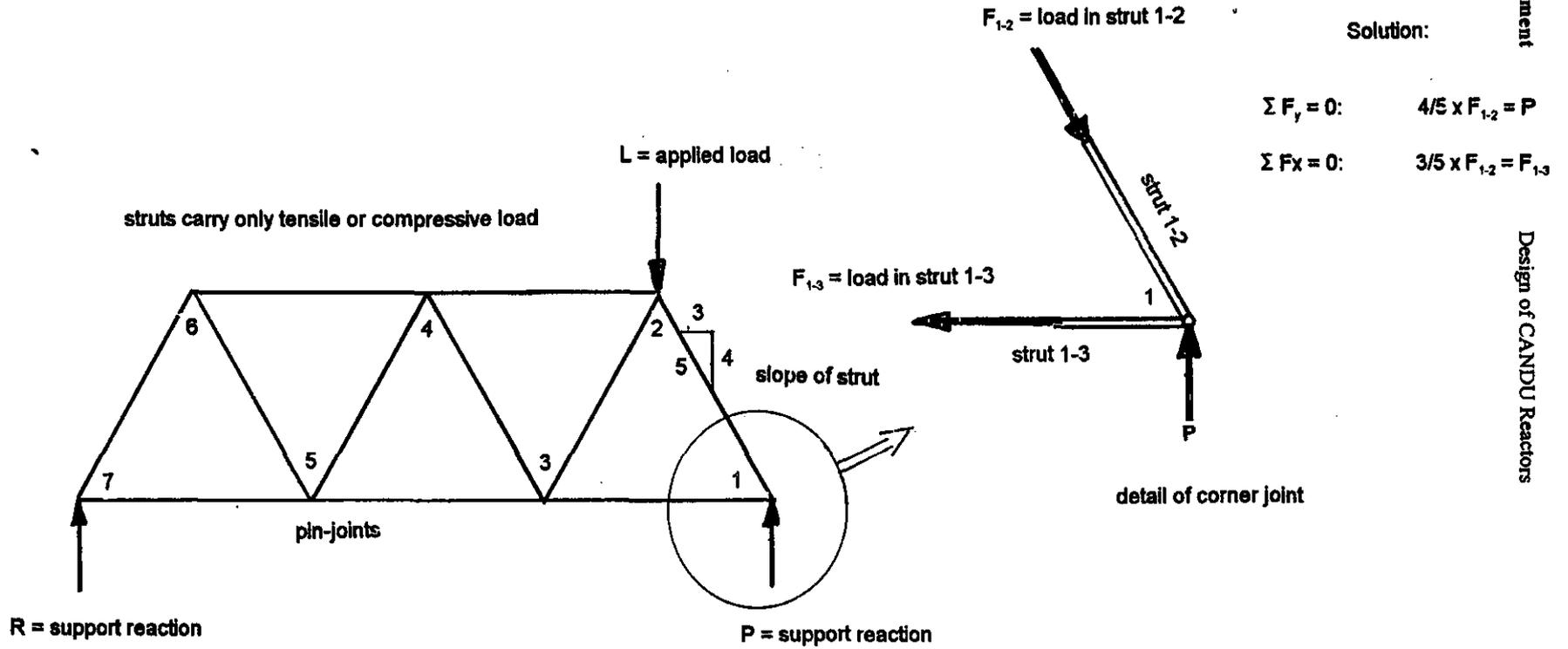
Figure 3-13 Simple Pin-Jointed Truss
