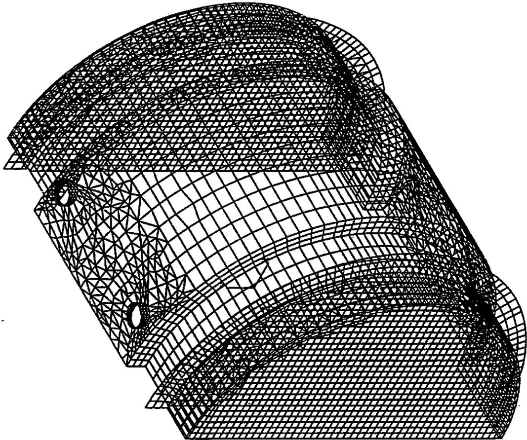
Figure 3-16 Finite Element Model for a CANDU Reactor Structure
