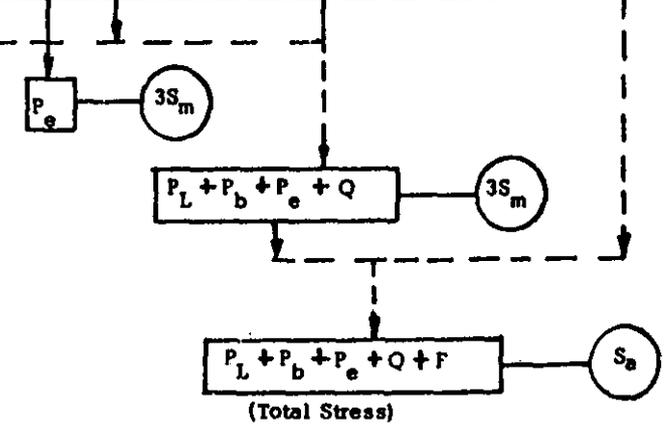
Figure 3-11 Allowable Stress Intensities for Normal & Upset Operating Conditions
