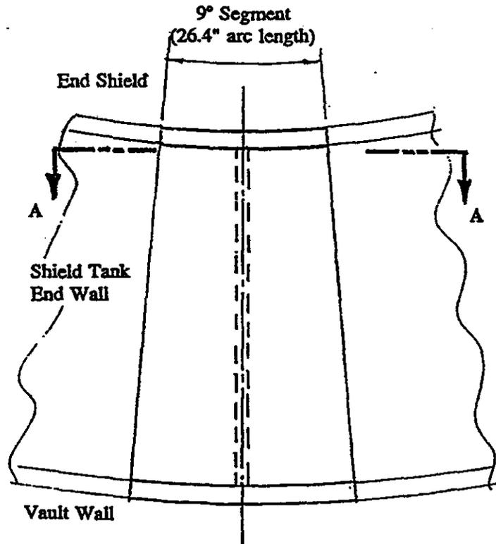
Figure 3-2 Section of Segment of Shield Tank End Wall used to Compare Edge Fixing Concepts
