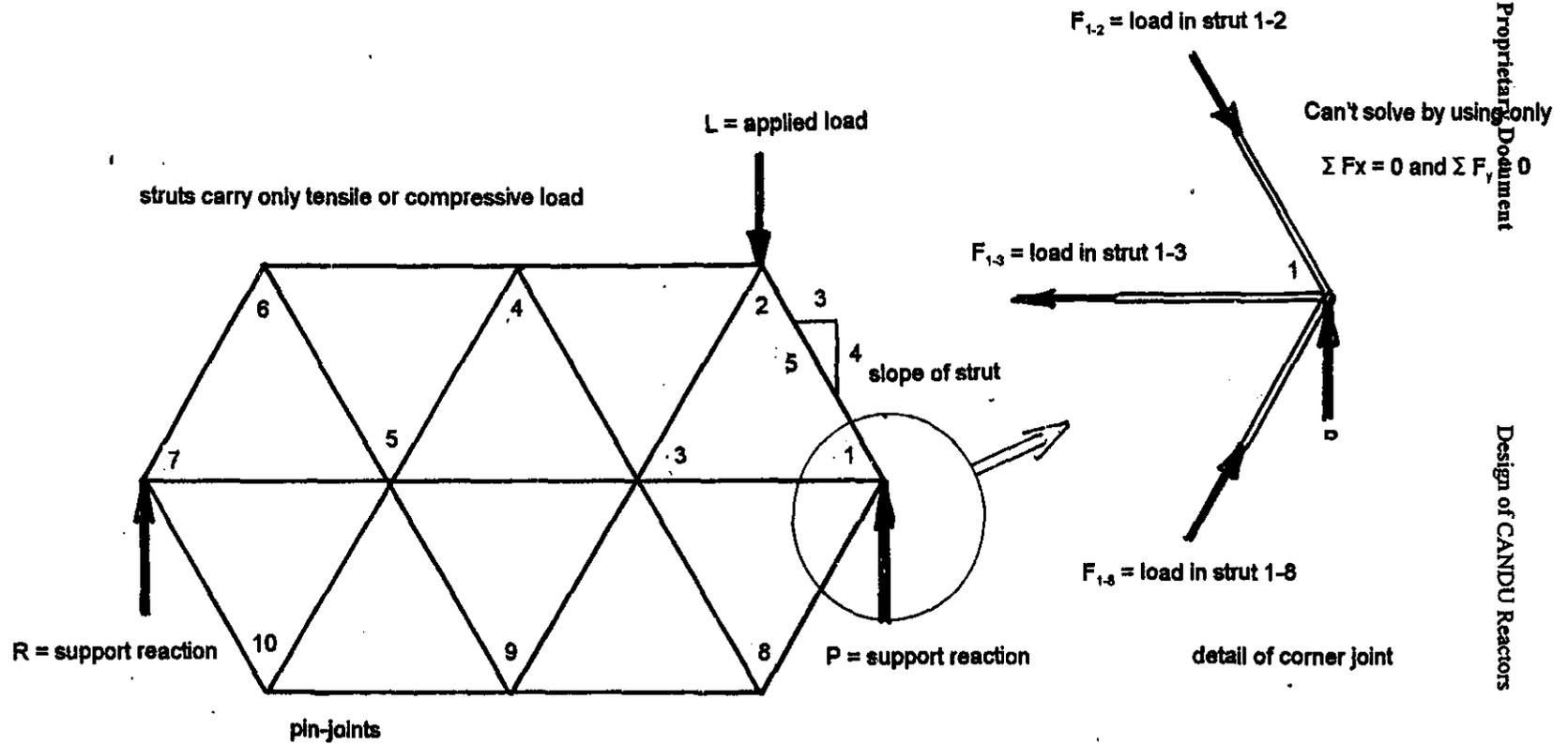
Truss is redundant because any strut can be removed and truss will still carry load
