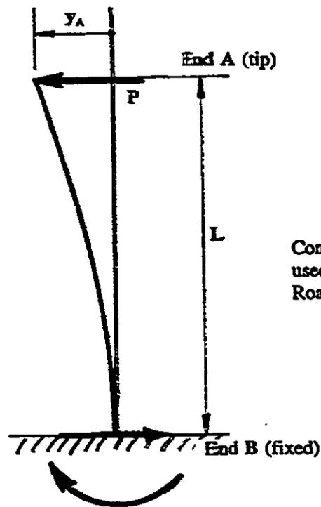
Convention of parameter identification used in Tapered Beam Equations in Roark, Table 13d, Case Ia, for  $a=0$ .
